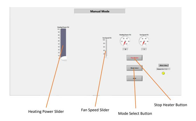
**Heating Power Slider:** Drag the slider to select the percentage of the maximum heating power. The output temp of the heat gun can be viewed on the heat gun's LCD. At maximum heating power, the heater coil temperature is 650 °C.
