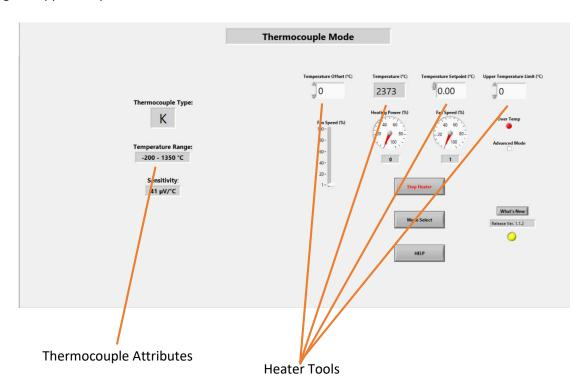
**Thermocouple Attributes:** Automatically shows the type, effective temperature range, and sensitivity of the selected thermocouple type.
