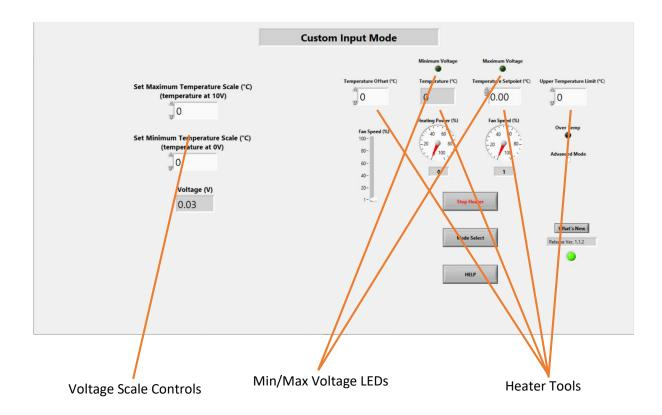
**Voltage Scale Controls:** Set the extremes of the temperature scale from your part. For example, if your part can read from -180 to 450 °C and these values correspond to 0V and 10V outputted by your part, respectively, and assuming the temperature scales linearly to voltage, enter in "-180" as the minimum temperature scale value and "450" as the maximum temperature scale value. The voltage value reads the raw voltage signal from the BNC connector.
