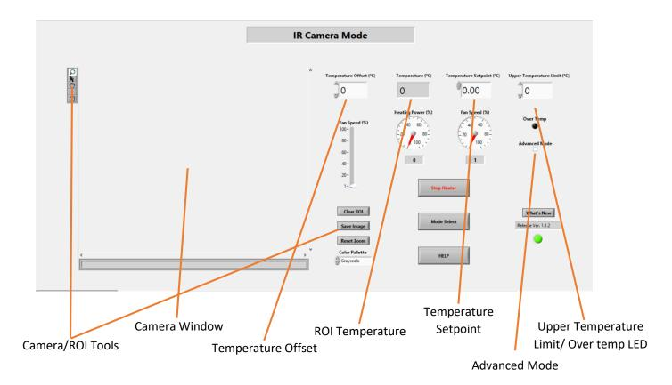
Camera/ROI Tools: Select which ROI type (point and box are currently available), then place the ROI in the camera window. You can also zoom, manipulate ROIs, and drag the image with the other ROI tools. The camera tools allow you to clear the selected ROI, reset the camera zoom to default, change the color palette, and save an image to the desktop (saves as "image.png" and overwrites itself every time the 'save image' button is pressed. Be sure to save or rename image.png every time).
